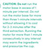
Friction from the rotating blade when extracting can cause ingredients to heat and generate internal pressure in the sealed vessel. If the vessel is warm to touch, allow to cool before carefully opening pointed away from your body.
